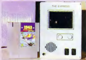
This early preproduction model of the portable Nintendo sported a clear color LCD, external control ports and full compatibility with NES carts!
